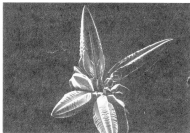
Figure 3. A hemispherical deposit structure of gold from LCVD with a stationary beam, obtained with 100-mW laser power on alumina with a beam diameter of approximately 10 \mu\text{m} .
